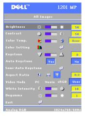
**BRIGHTNESS**—Use the  $\bigcirc$  or  $\bigcirc$  button on the control panel or the  $\blacktriangleleft$  or  $\blacktriangleright$  button on the remote control to adjust the brightness of the image.
