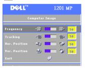
**FREQUENCY**—Change the display data clock frequency to match the frequency of your computer graphics card. If you see a vertical flickering bar, use Frequency control to minimize the bars. This is a coarse adjustment.
